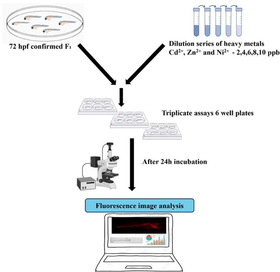
**Fig. 1.** Experimental Setup for Heavy Metal Detection Assay. Zebrafish F1 generation larvae at 72 hpf and free of structural deformities, ten larvae per well, in triplicate, were cultured in 6-well plates with, Each well received 3 mL of control (0 ppb) or varying concentrations (2, 4, 6, 8, and 10 ppb) of Cd<sup>2+</sup>, Pb<sup>2+</sup>, and Ni<sup>2+</sup> solutions and plates were then incubated at 28 °C for 24 h. Subsequently, larvae were examined under fluorescent microscopy.
