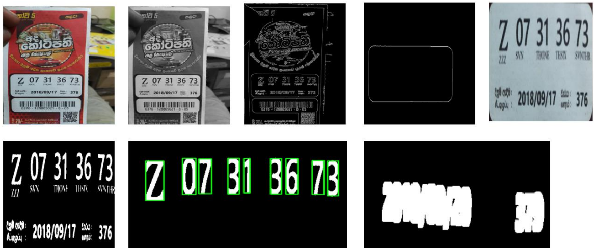
Figure 1 Above image shows the steps of image processing.
