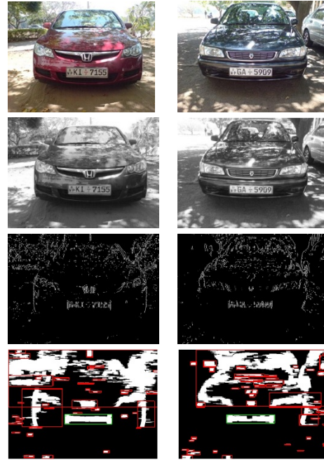
Fig. 3. Row 1: RGB images, Row 2: Grayscale images, Row 3: Detection of vertical edges, Row 4: Plate localization
