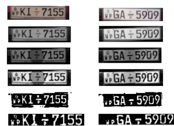
Fig. 4. Row 1: Plate regions extracted, Row 2: Rotated plates to align with the horizontal axis, Row 3: Top hat transformation, Row 4: Enhanced intensities, Row 5: Binary images, Row 6: Results obtained after applying the pre-processing algorithm-white characters in the black background.
